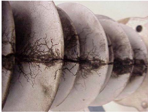
Fig. 3.21: Typical sample of tracking (and some erosion) on an outdoor insulator.
