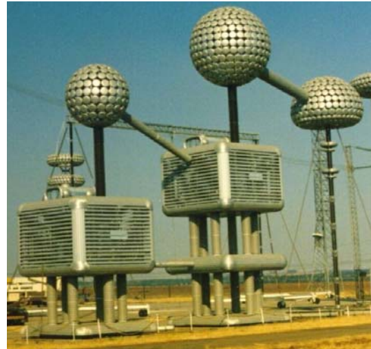
Fig. 4.3: Cascade connected test transformers
