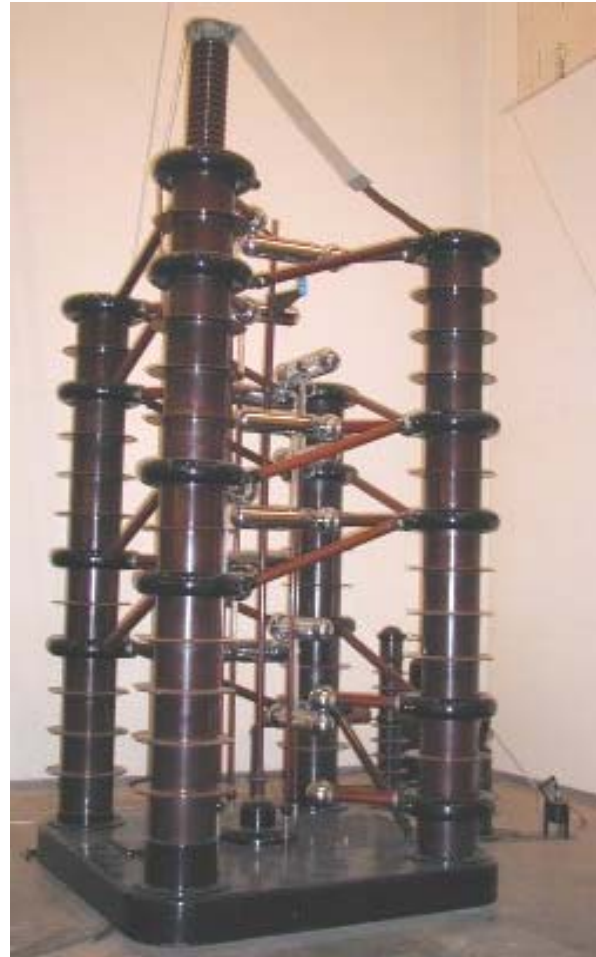
Fig. 4.10: 8- stage impulse generator
